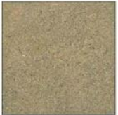
CONCRETE PAVING W/TOPCAST FINISH INTEGRAL COLOR
